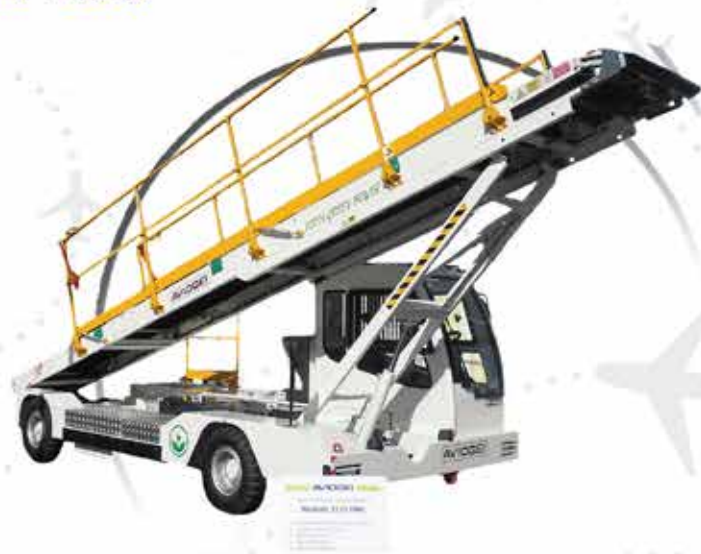
Conveyor Belt - NS450L Electric
