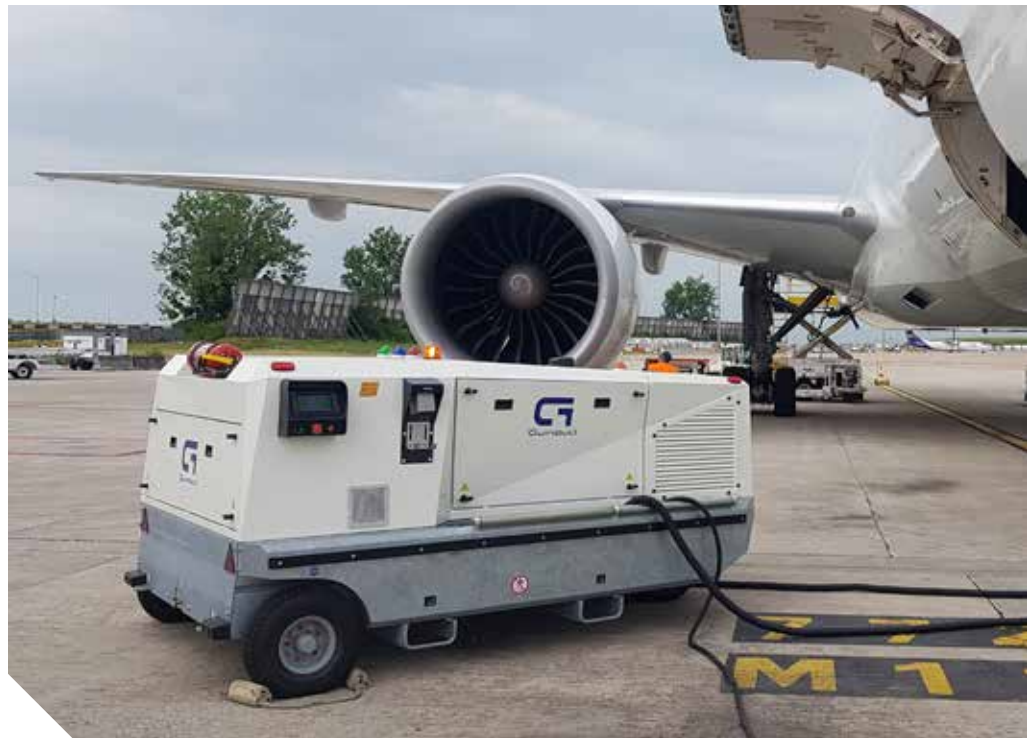
Guinault's EGA battery-powered GPU
