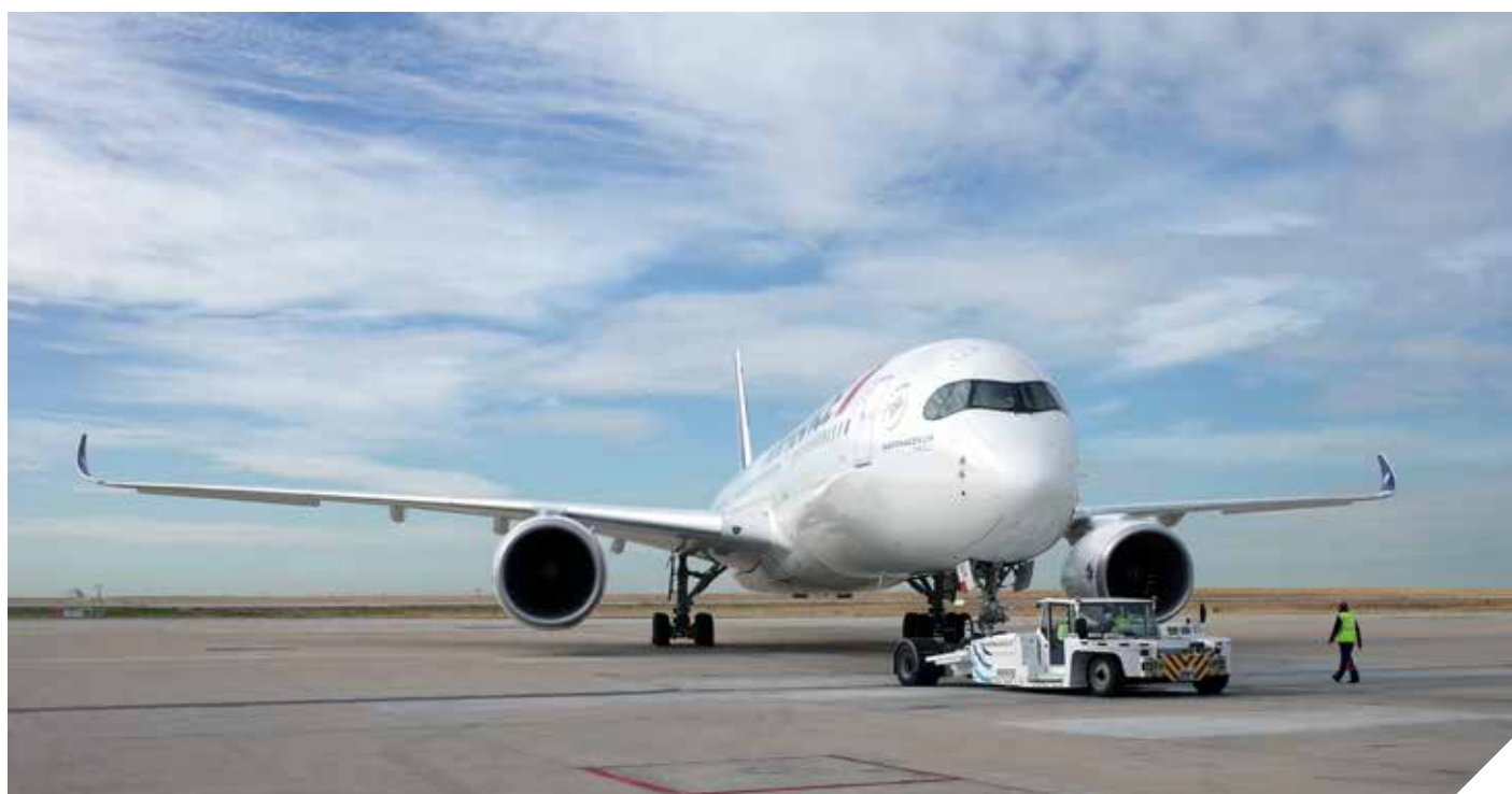
A TLD TPX-200-XE electric tug working with Air France at Paris Charles de Gaulle International
