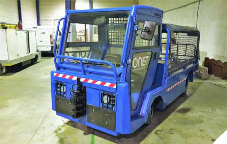
This Charlatte P2000 electric tractor has been refurbished and converted by ABC into a pushback/baggage cart for business jet operations
