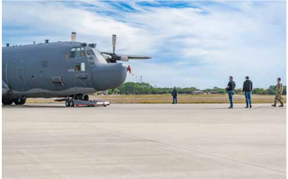
The TowFLEXX HD190 can pull aircraft the size of a Hercules, such as this C130H of the US Air Force
