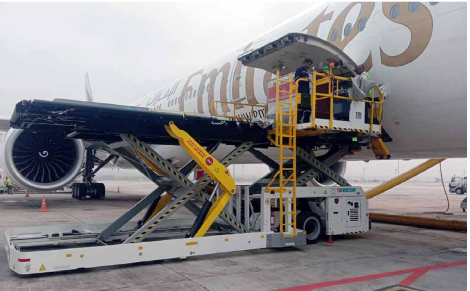
A fully electric TLD loader with the company's ipHS pluggable hybrid power pack technology
